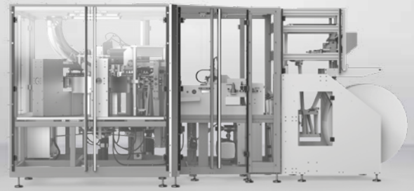
Mandrel wheel machine Production of flour and sugar packaging, 130 packs/min
